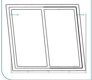
Once the window is in place, be sure to check that all Click-In fasteners have clicked into place. Make any adjustments with the fixed spanner (A).
