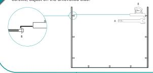
Rest the window at an angle on the base screws (or wooden/plastic washers) and tilt the window into place until you hear a "click" sound. Remember to place the window on the entire base first and then push the right and left sides in at the same time.
