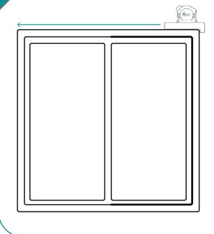
Place the locked tape measure (E) behind the screw head. If adjustments are necessary to fit the tape measure between the screws, adjust on the unlevelled side.
